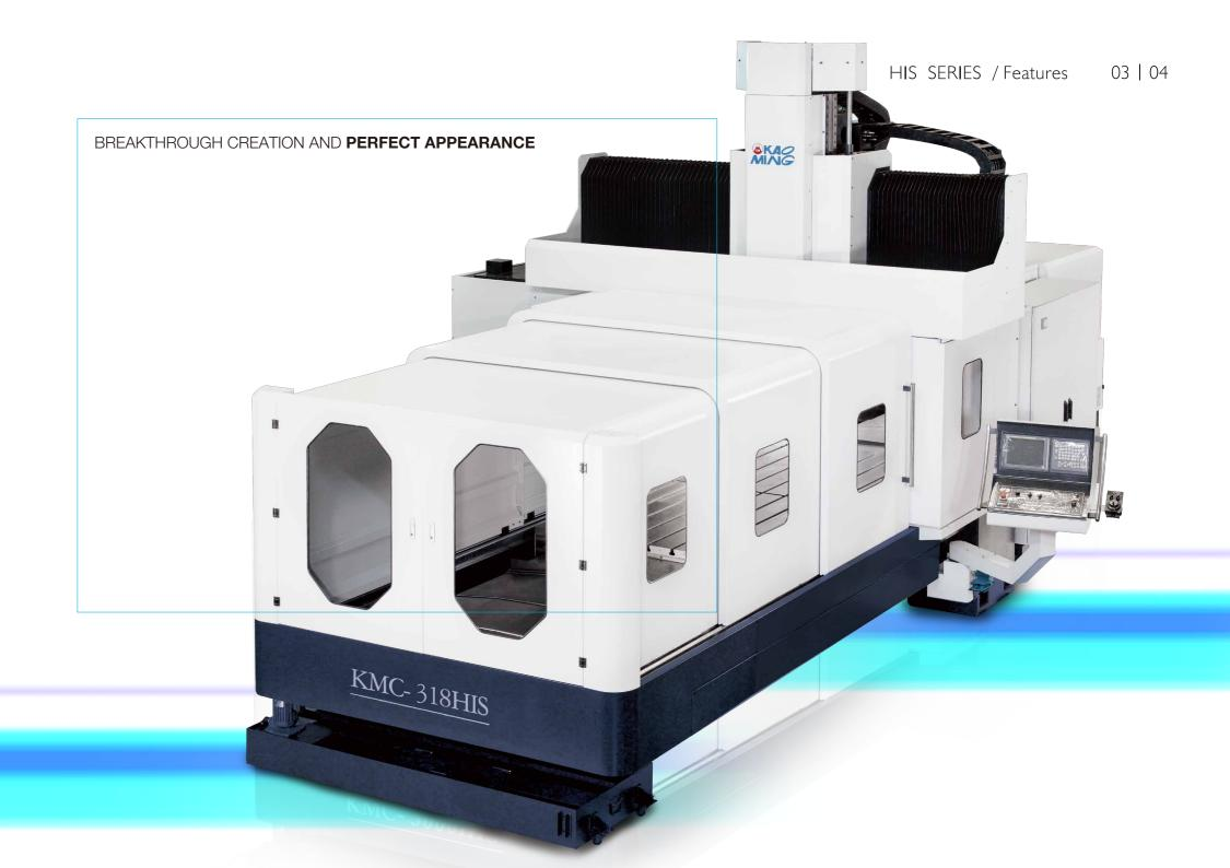
Tow column and crossbeam is of meehanite cast iron, after annealing to have internal stress relief can provides optimum bending and torsion stress, giving the best rigid structure.
